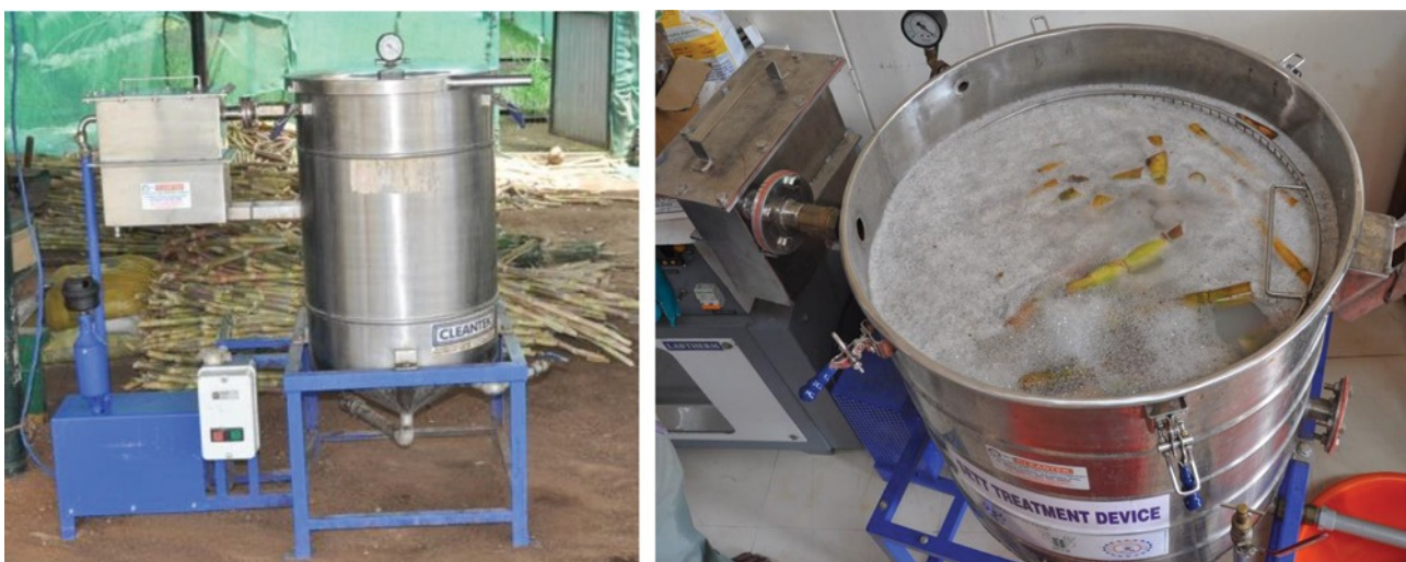
Figure 35. Mechanized sett treatment device to treat sugarcane setts with fungicides and other agro inputs. Left: View of the sett treatment device installed at Vellode, Erode District, Tamil Nadu, India; Right: Inside view of the device with setts dipped in the treatment solution.
