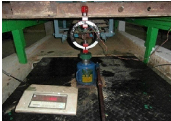
Fig. 2 Calibration of ring transducer for measurement of normal load
