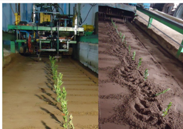
Figure 4: Soil bin profile before and after weeding operation.
