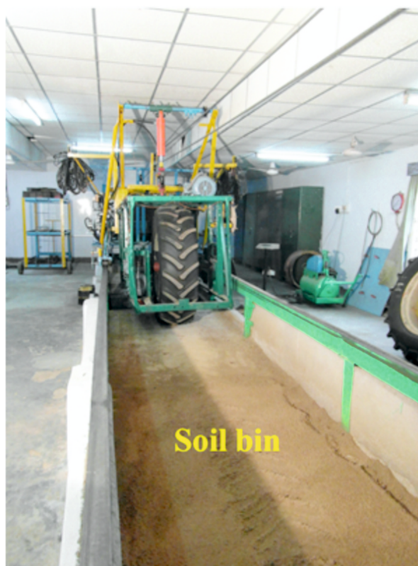
Fig. 3: Tyre test on soil bin
