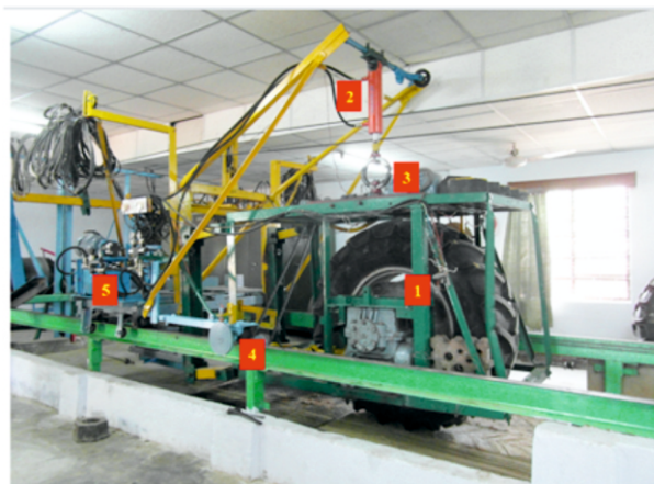
Fig.2: Constructional details of the tyre test carriage with hydraulic system
