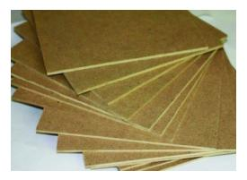
Fig.12: Cotton stalk particle boards
