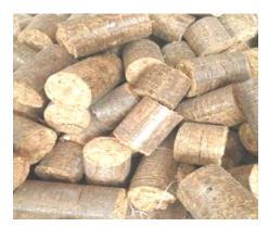
Fig. 6: Cotton Stalk briquettes
