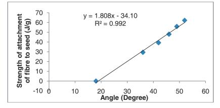
Fig 3. Calibration of SDL 2 fibre seed strength of attachment tester
