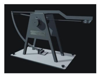
Fig 1. Cotton fibre seed attachment tester
