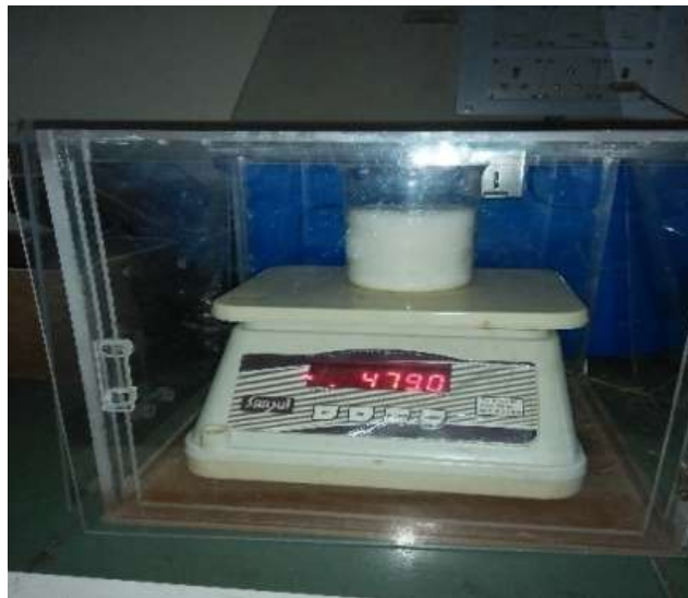
Fig.2 Measurement of bulk density
