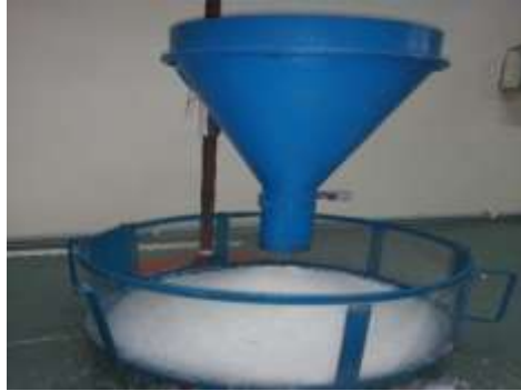
Fig.4 Measurement of coefficient of friction
