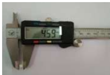
Fig.6 Measurement of average urea grain diameter
