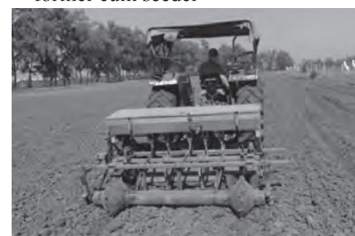
Fig. 5 Developed rotary assisted bed former cum seeder
