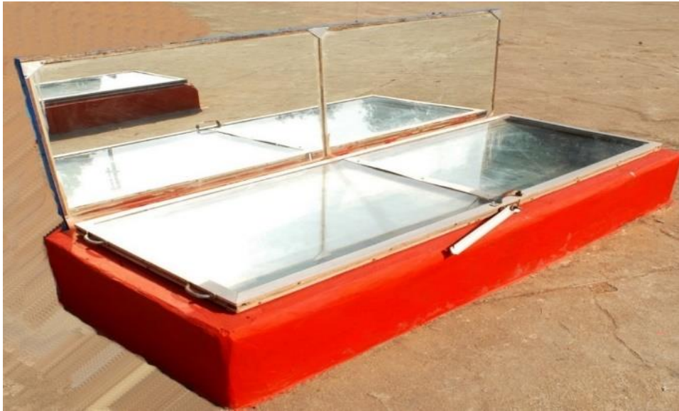
Fig.11. Solar cooker for animal feed with reflector
