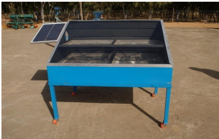
Fig.8. PVT hybrid solar dryer installed at CAZRI solar yard
