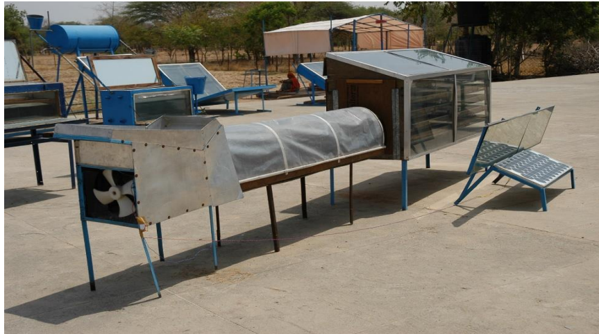
Fig. 6. PV winnower cum solar dryer
