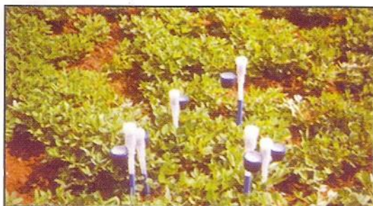
Photo.12: Measurement of soil upland flux under shallow water tables situation.
