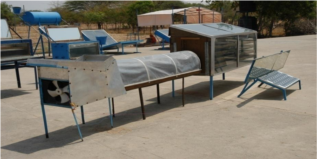
Fig. 1: PVT hybrid solar dryer with winnower installed at CAZRI solar yard
