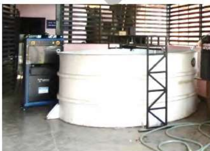
Fig. 4 Moving gantry system installed at ICAR-CIFT for studying swimming speed of fish
