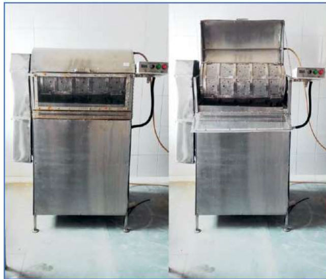
Fig. 5. Fish de-scaling machine with variable drum speed
