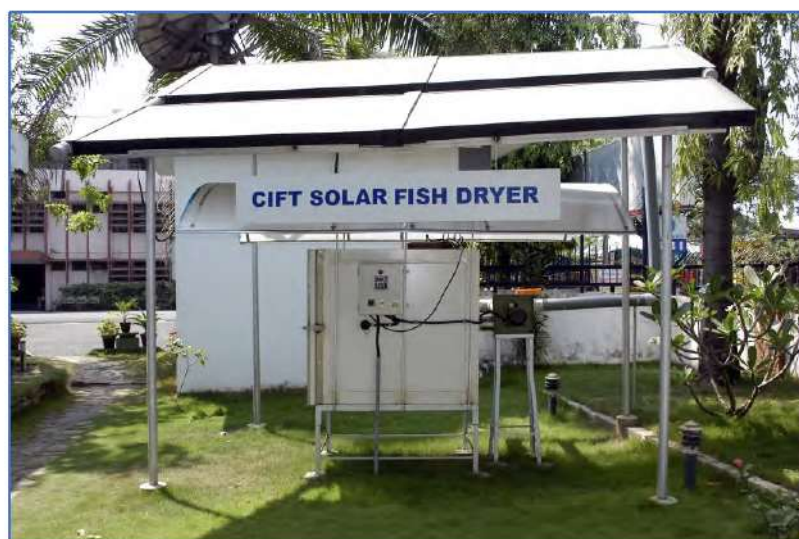
Fig. 2. ICAR-CIFT Solar-electrical hybrid dryer
