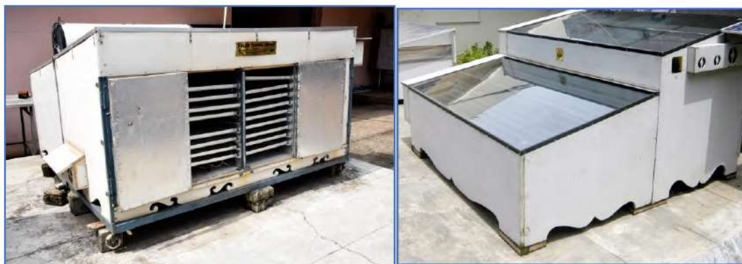
Fig. 3. ICAR-CIFT Solar- electrical hybrid dryer
