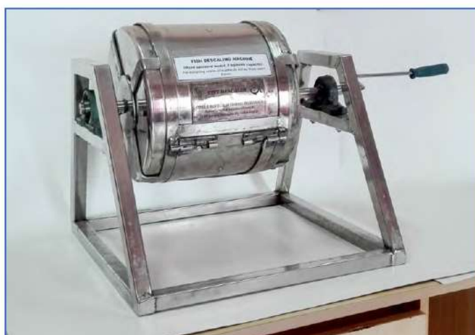
Fig. 7. Hand operated fish de-scaling machine
