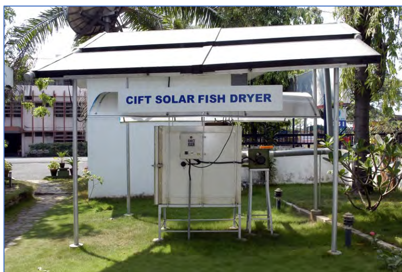
Fig. 2. ICAR-CIFT Solar-electrical hybrid dryer
