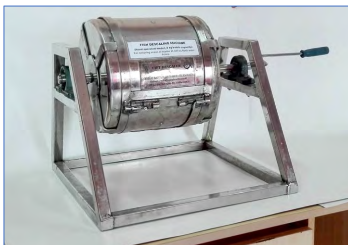
Fig. 7. Hand operated fish de-scaling machine
