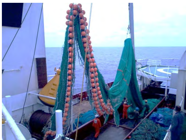
Fig.7 49.5m Krill trawl
