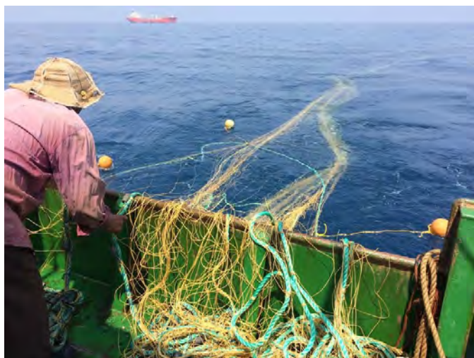
Fig.2 UHMWP trawl under operation
