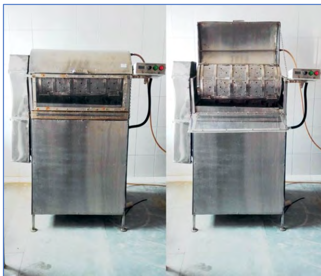
Fig. 5. Fish de-scaling machine with variable drum speed
