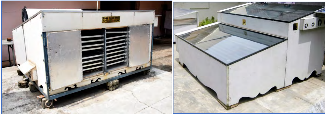
Fig. 3. ICAR-CIFT Solar- electrical hybrid dryer
