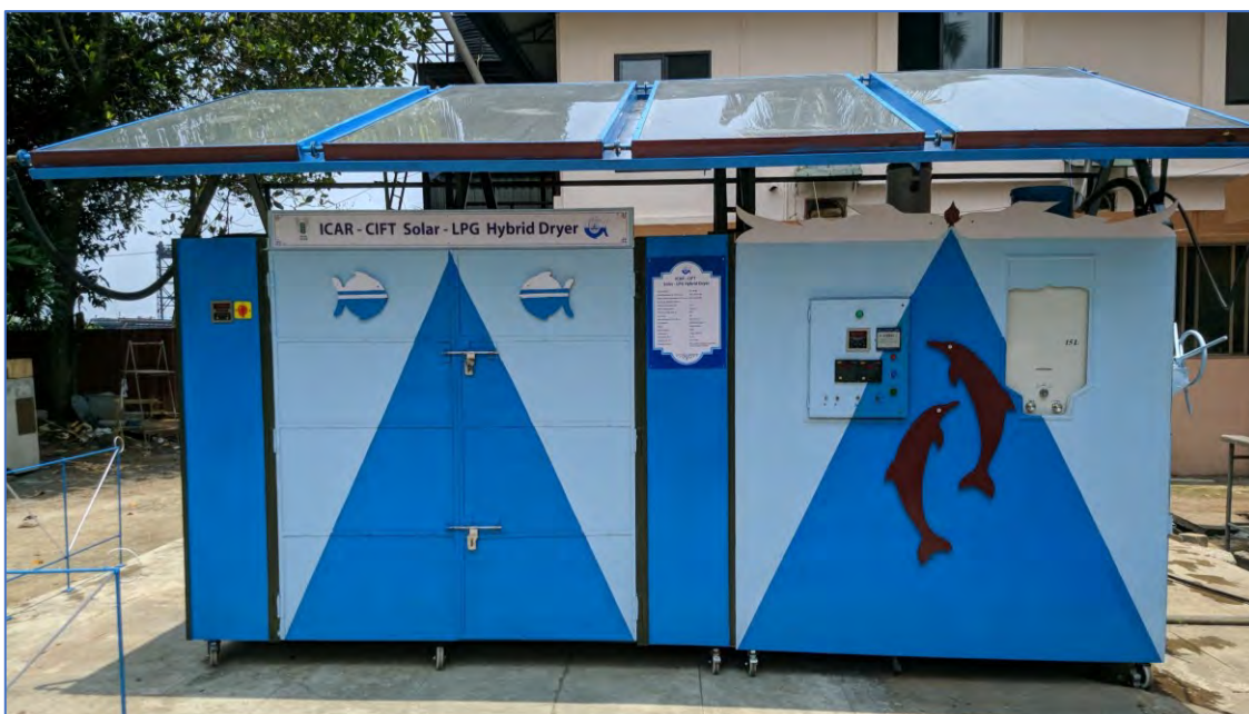
Fig.1. ICAR-CIFT Solar-LPG hybrid dryer
