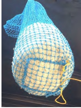
Fig.11 Square mesh codend with base panel
