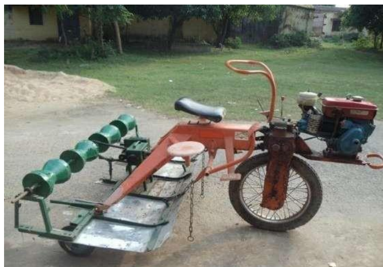
NRRI Eight row self-propelled seeder
