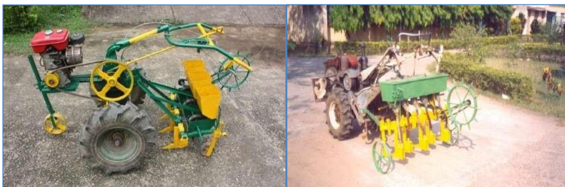
NRRI three row hill seeder & multi crop seed drill
