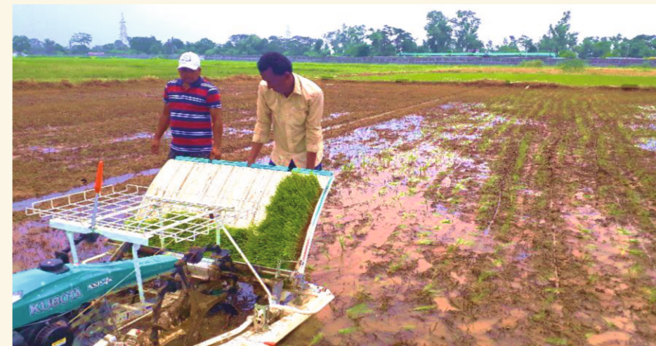
Fig. 3(a) Mechanised transplanting with walk-behind type transplanter
