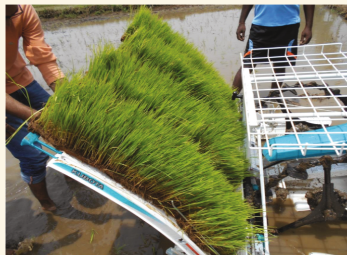
Fig 2. Seedlings on mat nursery placed on transplanter for transplanting
