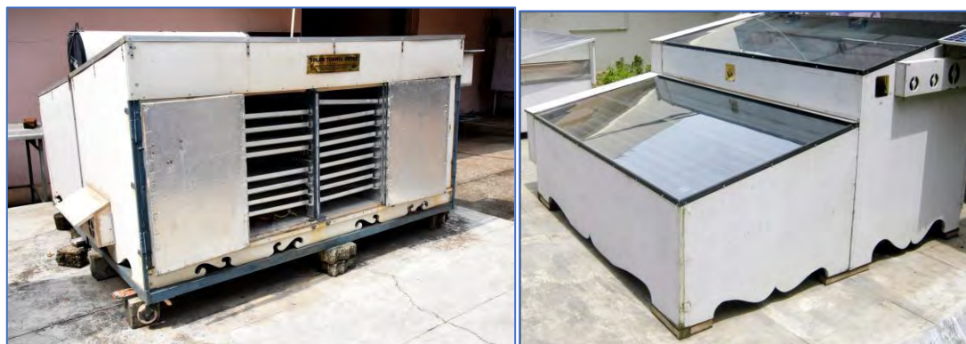
Fig. 3. ICAR-CIFT Solar- electrical hybrid dryer
