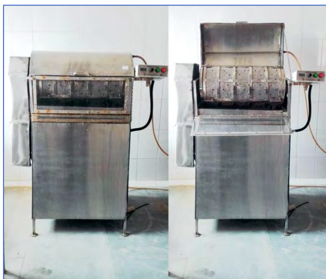
Fig. 5. Fish de-scaling machine with variable drum speed
