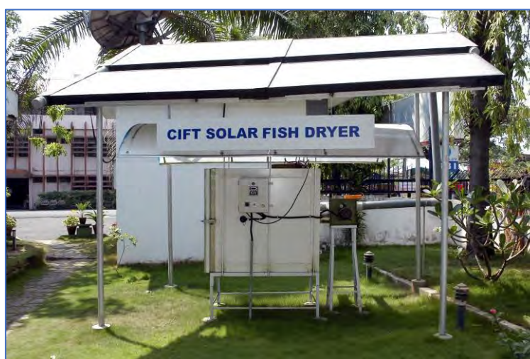
Fig. 2. ICAR-CIFT Solar-electrical hybrid dryer
