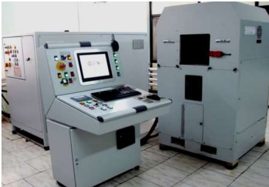
A Research model of 2 litre capacity High Pressure machine from M/s Stansted Fluid Power Ltd, United Kingdom at Central Institute of Fisheries Technology, Cochin.
