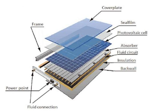
cell converts the photons which present in solar rays to direct-current (DC) and voltage. A single PV device is known as a cell. An individual PV cell is usually small. These cells are made of different semiconductor materials and are often less than the thickness of four human hairs. A single PV cell typically produce about 1 or 2 watts of solar electric power.
