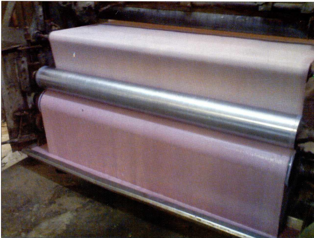
Fig. 7. Adhesive Bonding of Textile Reinforcement
