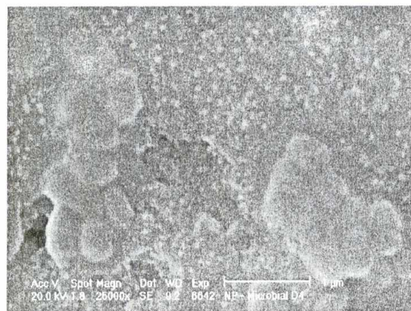
Fig. 10. SEM Image of Nanocellulose Prepared by the Fungus, Trichoderma reesei (Scale bar = 1 μm)
