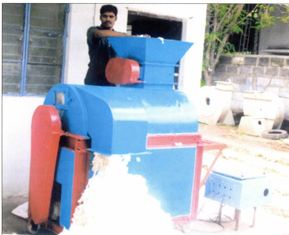
Fig. 4. Fabricated set-up of an Axial Flow Cotton Precleaner
