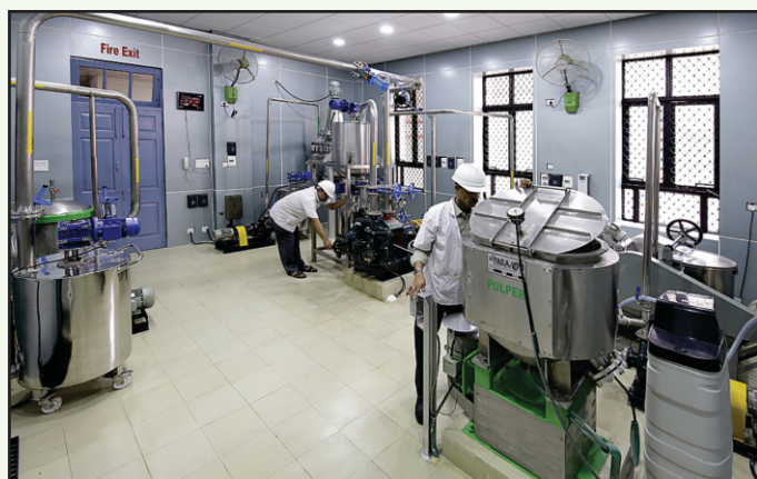
Refining unit for production of Nano Cellulose
