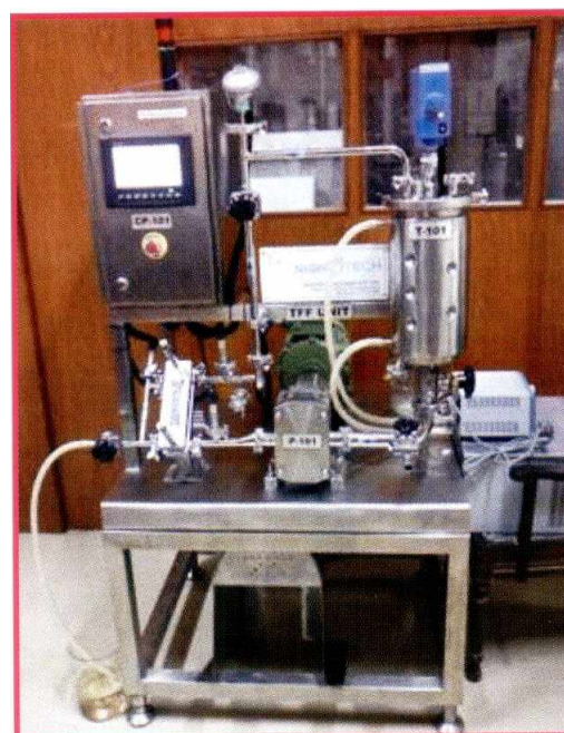
Photograph of membrane bioreactor
