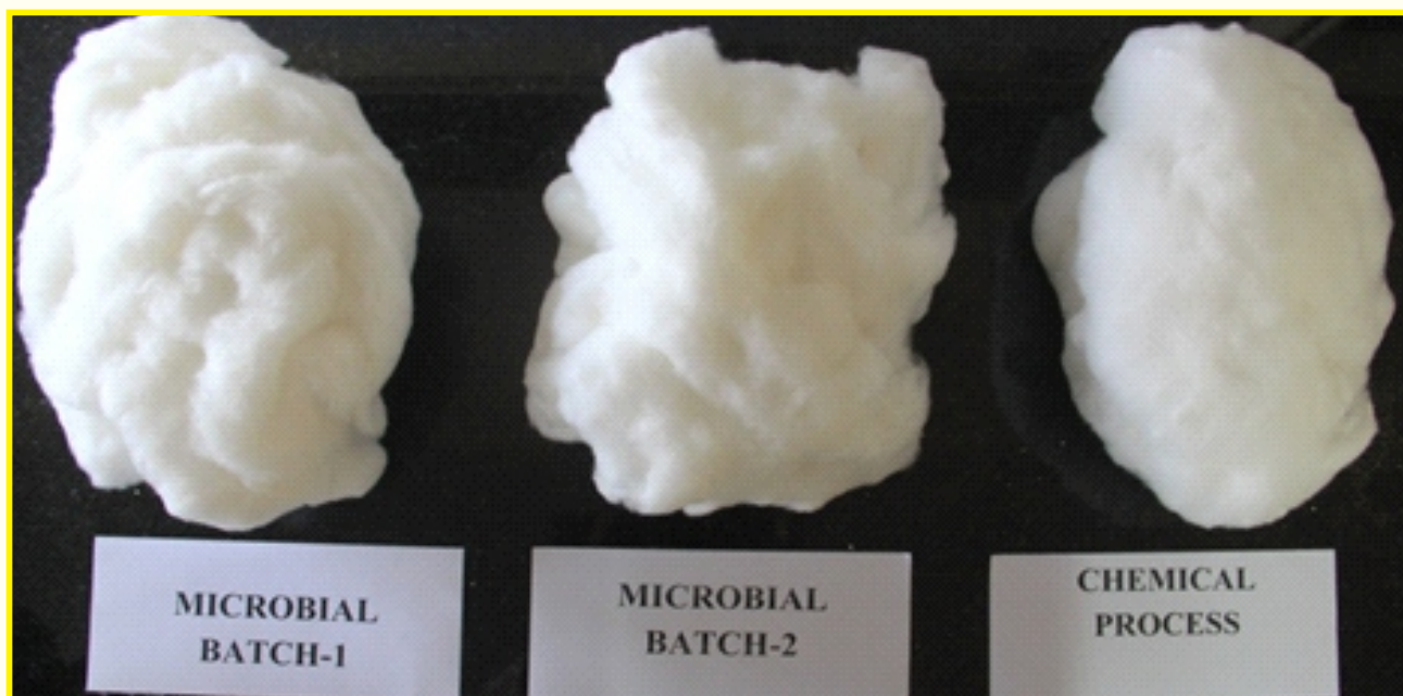
Photographs of absorbent cotton prepared by microbial and chemical routes
