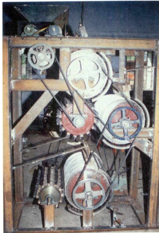
Cotton Stick Removing Machine — An Internal View
