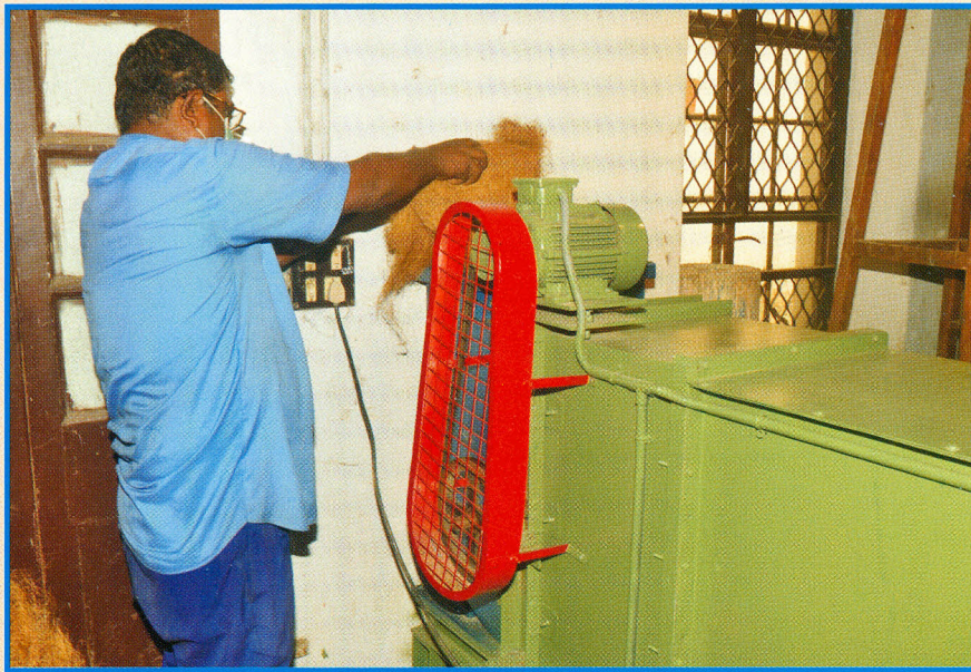
Fig. 1 : Fibre Feeding to the Machine
