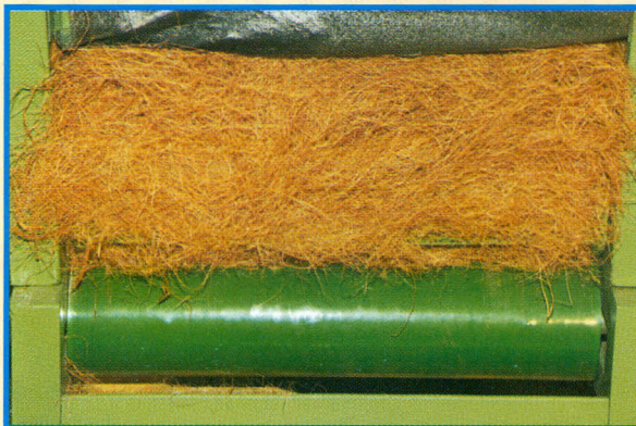
Fig. 2 : Coarse Fibres Collected on Conveyor Belt
