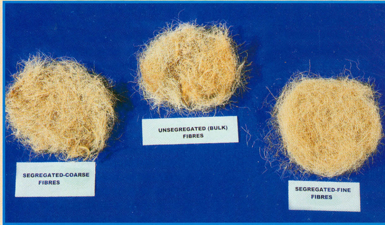
Fig. 4 : Unsegregated and Segregated Fibres
