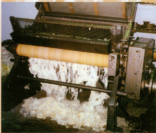
Fig. 4 Self-grooving rubber roller in operation
