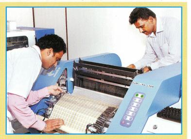
sample production and can produce samples of 20 inches wide by three metres long, with low wastage of expensive yarns.
