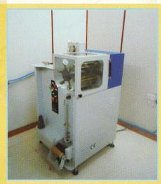
**Sizing Tank:** Electricalheating with electronic controls and tank is detachable for cleaning
