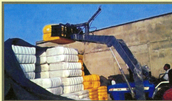
Mechanical Bale handling system
