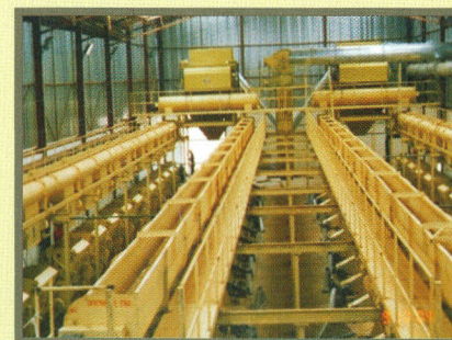
Automatic Individual Seed Cotton Feeding System to Gins (4 rows)
