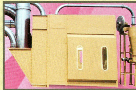
Primary and secondary filters in compactor in dust control equipment
