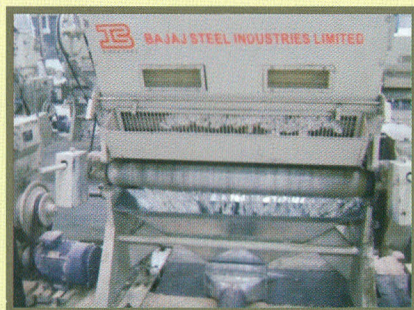
DR Gin with Autofeeder and Lint collection system
