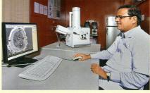
Scanning Electron Microscope (SEM)
