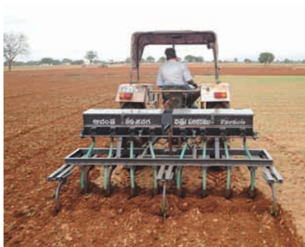
Sowing of groundnut using tractor drawn Ananta planter (left) and field view of groundnut (right)
