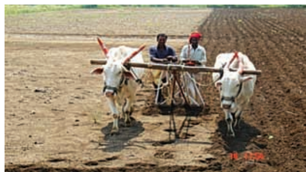
Sowing of rabi sorghum with two bowl ferti-seed drill
