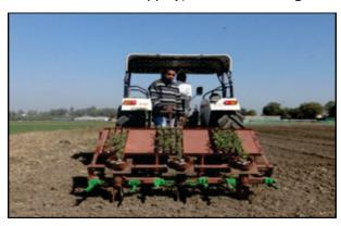
(disc type), seedling tray shifter, seedling trays, ground wheels and chain and sprocket type power transmission system. The average field capacity, field efficiency, labour requirement and fuel consumption of transplanter are 0.11 ha/h, 56%, 18 man-h/ha, and 3.5 l/ha, respectively; whereas, transplanting efficiency and overall efficiency are 92% and 85%, respectively, for tomato and chilli seedlings at the forward speed of 1.2 km/h.
