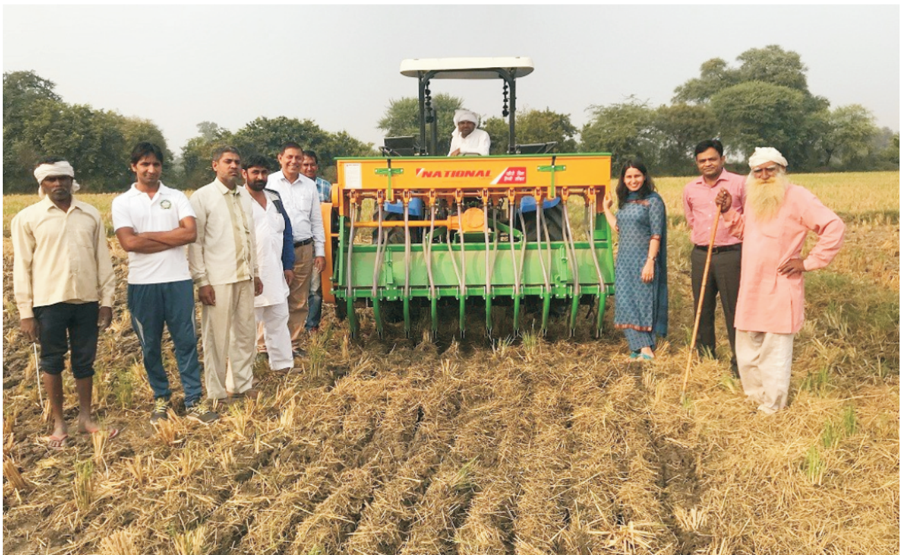
Zero till wheat sowing by happy seeder
