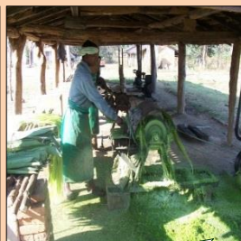
Extraction Fibre from sisal leaf
