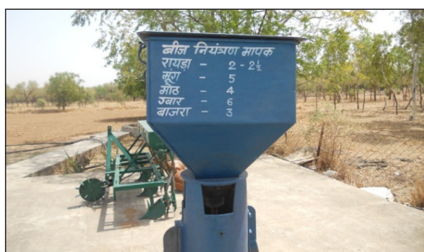
Fig. 2. Seed rate marked on seed box.
