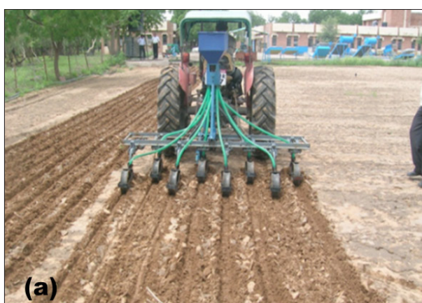
Fig. 3. Sowing by improved traditional seed drill (a) and sowing by traditional seed drill (b).
