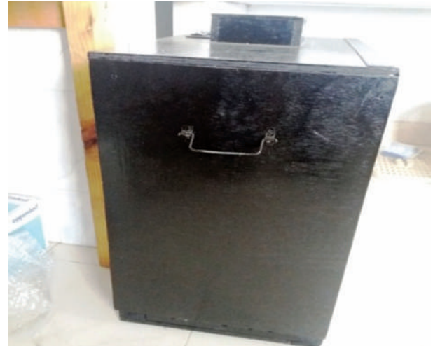
Side view with double walled insulation with handle on both sides for easy carrying
