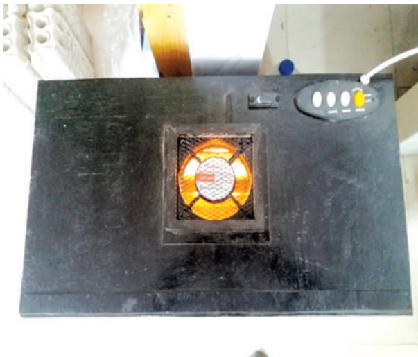
Top view with heat control panel and air outlet with provision of net covered axial fan.
