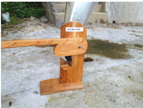
Lateral view humane killing cone with adjustable knob for different bird size
