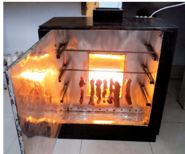
Inner view with aluminum coating. Two layered net protected 3 halogen tubes of 400 watt each at the back. Lateral walls with provision for 3 trays or rods with multiple hooks
