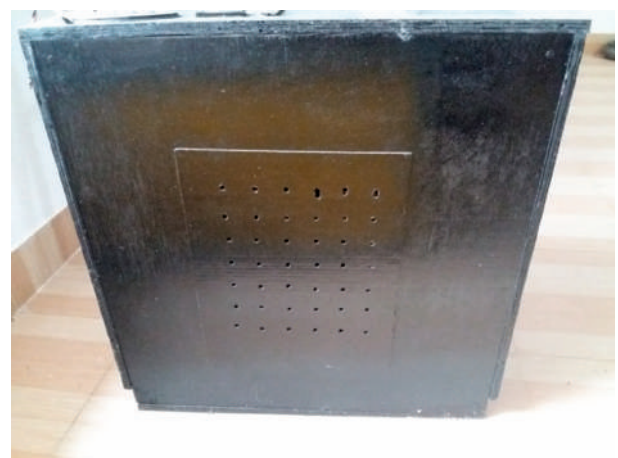
Heat outlet system at rear with double wall insulation
