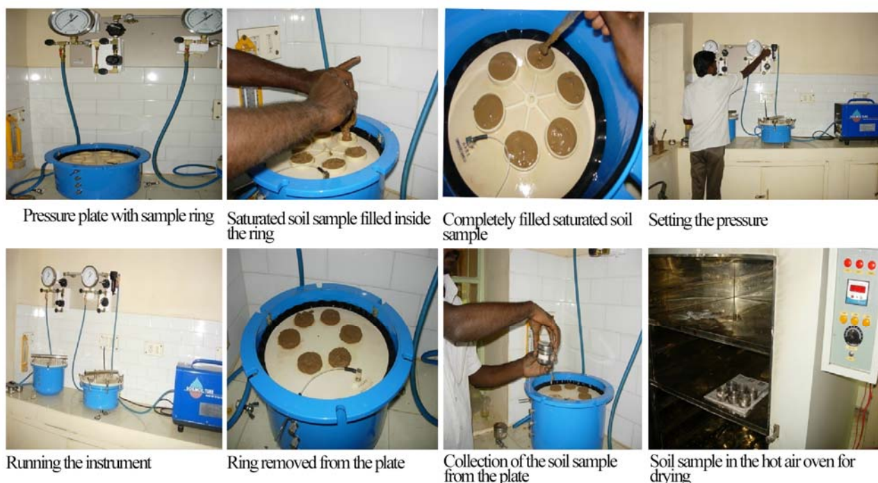
Figure 2 Soil moisture measurement by using Pressure Plate Membrane Apparatus
