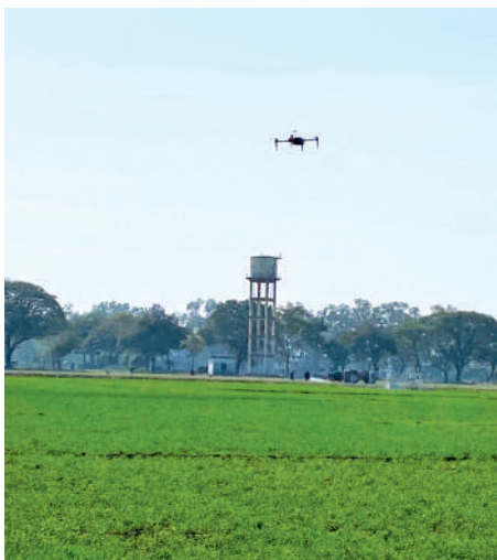
Fig. 5. Drone with multispectral camera for irrigation scheduling
