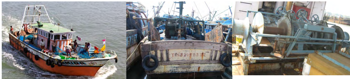
Fig.6 Commercial Trawler, otter boards seen hanging on the gallows and winch in the last
