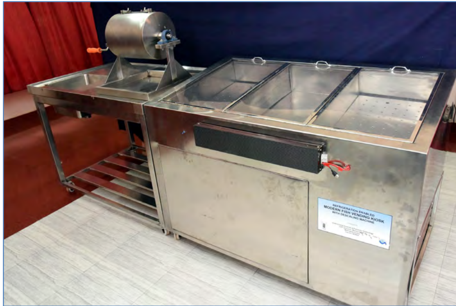
Fig. 8. Refrigerated mobile fish vending kiosk
