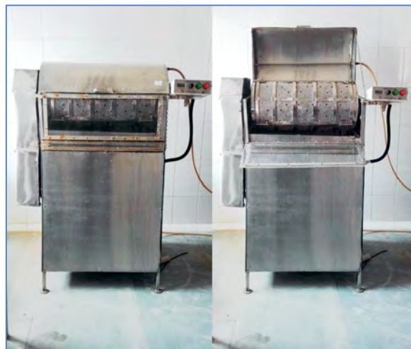
Fig. 5. Fish de-scaling machine with variable drum speed
