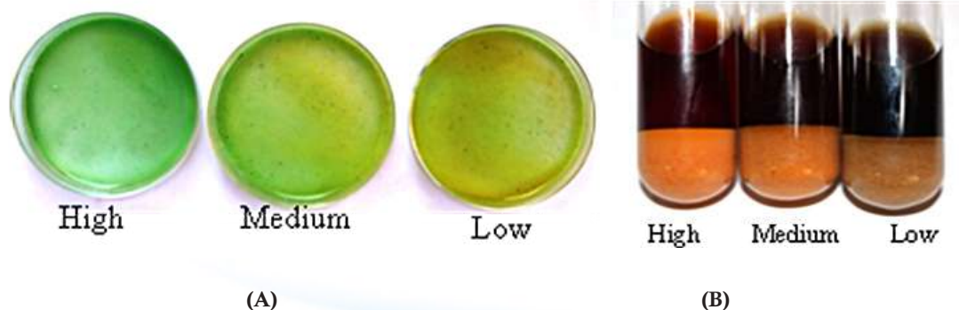
Rapid iron screening by Prussian Blue (A) and Zinc by DTZ (B) staining
