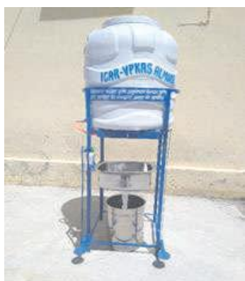
Fig.3.3.2. Foot operated hand sanitizer device
