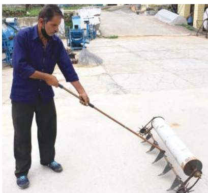
Fig. 3.31. Prototype of Manual Operated VL Multi-crop Sowing Device
