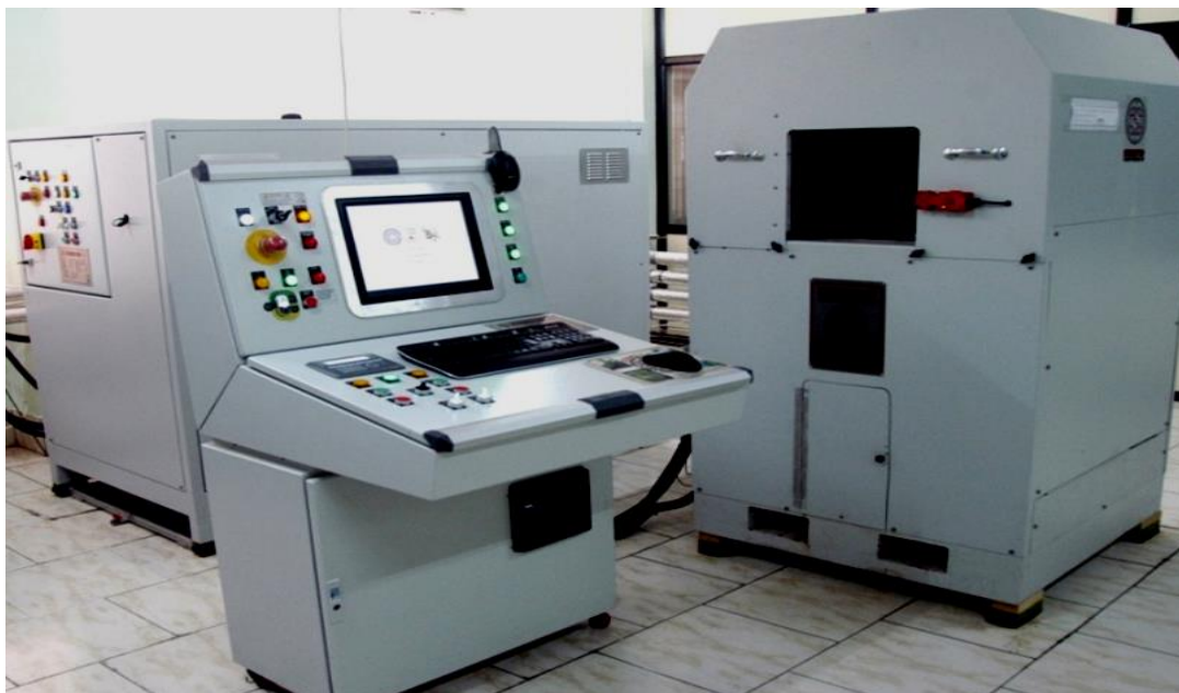
Fig.: A Research model of 02 litre capacity High Pressure machine at Central Institute of Fisheries Technology, Cochin (from M/s Stansted Fluid Power Ltd, United Kingdom)
