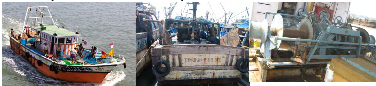
Fig.6 Commercial Trawler, otter boards seen hanging on the gallows and winch in the last
