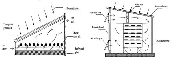
(a) Passive solar dryer (Grabowski and Mujumdar, 2000) (b) Active solar convective dryer (Imre, 1995)
