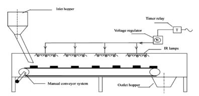
Conveyor type IR drying system (Ratti and Mujumdar, 1995)
