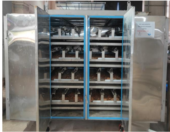
Fig. 3 Hot air-assisted continuous infrared dryer
