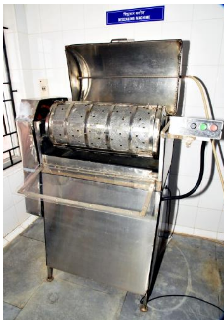
Fig.1 Fish de-scaling machine with variable drum speed
