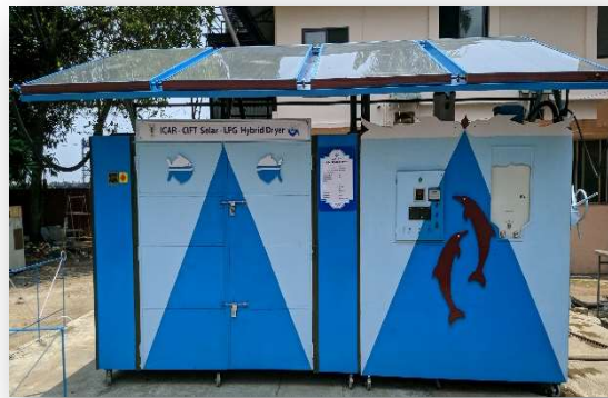
Solar dryer with electrical back-up
