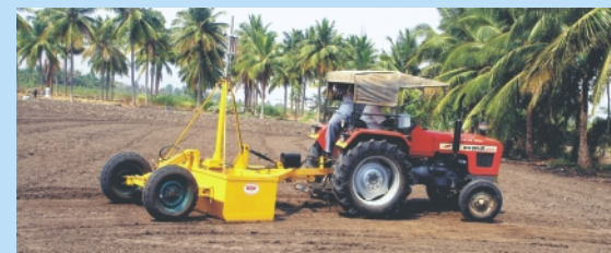
Laser leveller demonstration at Athipalayam
