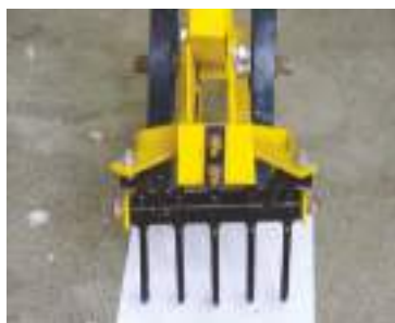
Photo 9. Modified CRIJAF nail assembly having 8 mm diameter nails with threads to fit with nail assembly bar by nuts and bolts
