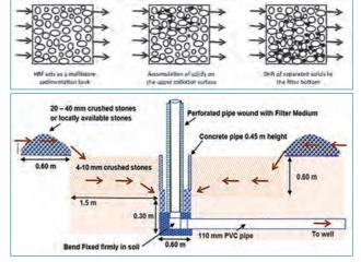
crushed or locally available stones and lower layer of the filter inside a pit of 0.6 m depth has 4-10 mm crushed stones. At the centre of the filter, nylon screens are wound over a vertical collection pipe, through which water passes. The filtered water is then conveyed to the open well for recharge. The filter is 1.8 m in radius and 60 cm in depth. Depth at the centre of the filter is 90 cm. The filter is installed in bare soil. The filter was
