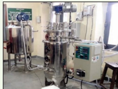
Fermentor and Mixing Tank
