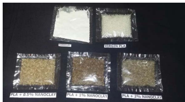
Virgin PLA, nanoclay and extruded granules of PLA/MMT in different concentrations
