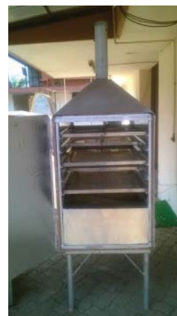
Small prototype of dryer with electrical backup
