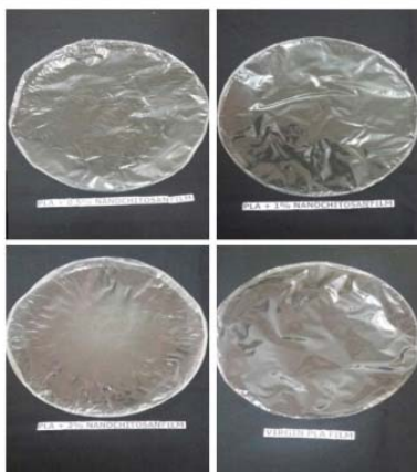
Virgin PLA and PLA/nanochitosan cast films in different concentrations
