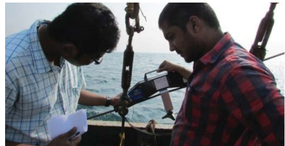
Onboard experimentation using tension meter
